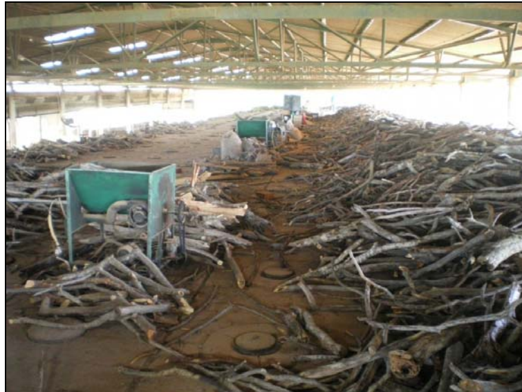
Figure 5. Mechanic burners and biomass utilized on the "Hoffman" kiln
