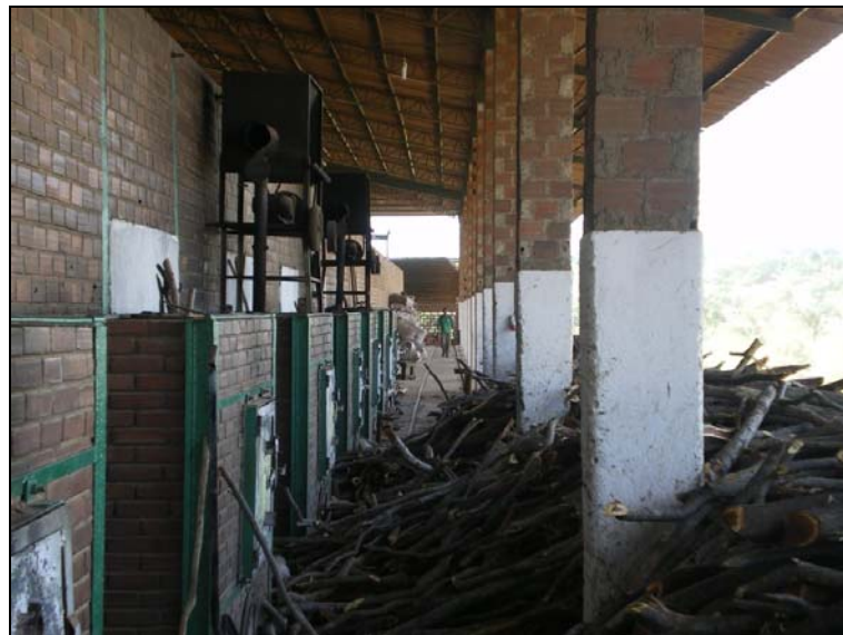
Figure 6. Mechanic burners and biomass utilized at the "Tunnel" kiln
