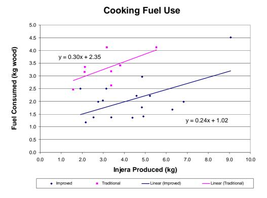
As can be seen from Figure 1, fuel use for the improved stove is substantially lower than for the traditional stoves. There is substantial variability, but the difference is large enough to be measurable with confidence on average. For typical cooking amounts relevant to this verification report (in the range of 3 to 4 kilograms of injera produced per cooking session), the fuel savings is slightly greater than 1.5 kilograms of wood per cooking session on average.
